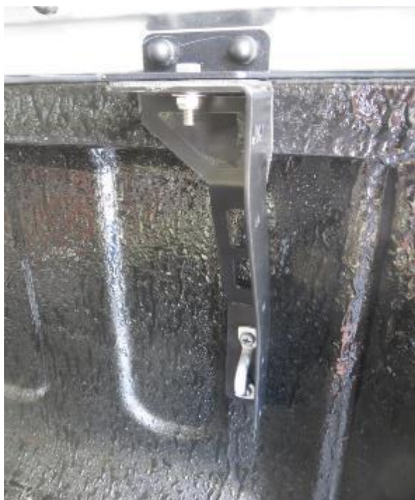
Figure 18: Rear-Right Support Bracket Installed
