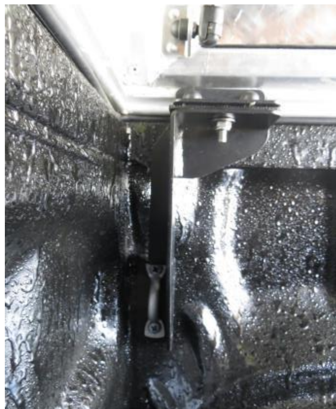
Figure 21: Front-Right Support Bracket Installed
